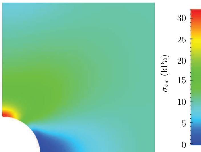
Figure 2.19:  $\sigma_{xx}$  stress field in the plate with hole.
